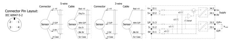
Putting Into Service: The sensor must be used with a galvanic isolation barrier designed to supply the sensor with a nominal 5V and to transmit the sensor output to a safe area. The barrier parameters must not exceed:
